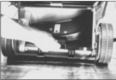
Figure 2 - Installing the Mulch Plug - 50m, 51m, 60m, 61m & 80m
